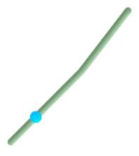
A linestring with the interpolated point at 20% position (0.20)
