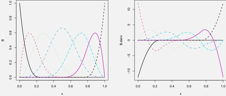
To summarize, in this illustration we have an order  $m = 4$  (degree = 3) B-spline (left) with 4 sub-intervals (segments) using uniform knots ( $N = 3$  interior knots, 5 knots in total (2 endpoint knots)) and its 1st-order derivative (right). The dimension of  $B(x)$  is  $K = N + m = 7$ .
