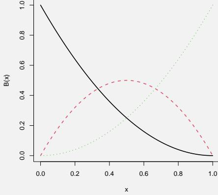
These bases are  $B_{0,2}(x) = (1-x)^2$ ,  $B_{1,2}(x) = 2(1-x)x$ , and  $B_{2,2}(x) = x^2$  and illustrate the foundation upon which the Bézier curves are built.
